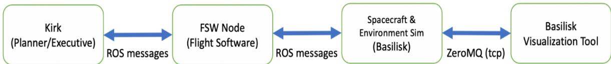
**Fig. 5. Demonstration pipeline showing interactions between components of the software prototype.**
