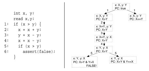
Figure 2. Code for swapping integers and corresponding symbolic execution tree.
