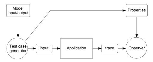
Figure 1. Test case generation and runtime verification.
