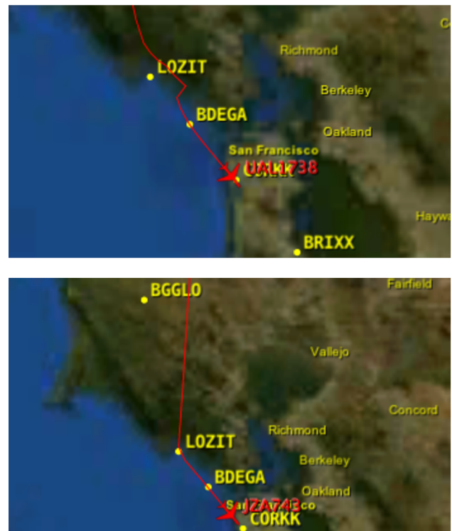
Fig. 8 Flight deviation from the assigned RNAV STARs detected at SFO
